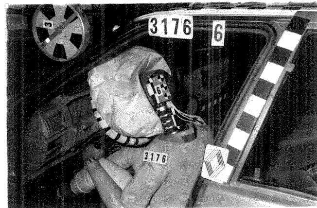
Figure 3. Static Deployment of COVER's Airbag: Out of Position Test
