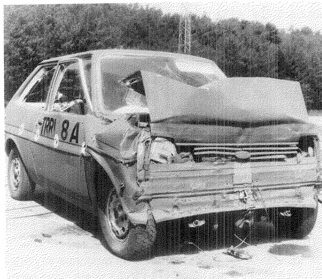
Figure 4. Full Width Perpendicular Block Impacted Car, Showing Uniform Deformation
