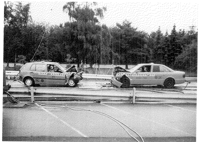
Figure 20. Frontal Crash Test Between Cars of Different Sizes (50 kph) (30 mph)
