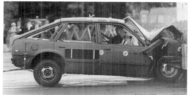
Figure 2. Perpendicular Rigid Block Impact, at 60 km/h, Showing Little Intrusion
