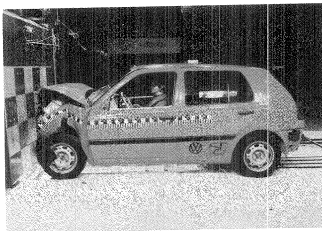
Figure 13. Frontal Impact Test at 56.3 kph (35 mph)
