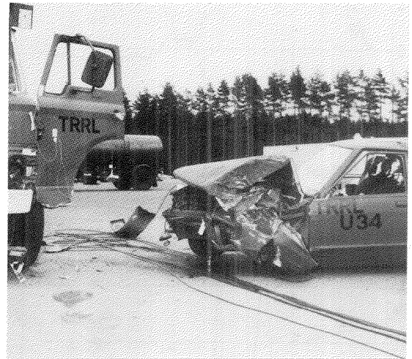
Figure 4. Test No. 4—Ford Granada, Underrun Guard Fitted to Truck
