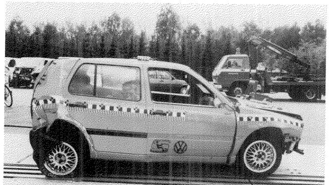
Figure 21. Rear Crash Test with 1800 kg Moving Barrier (48.3 kph) (30 mph)
