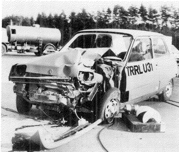
Figure 2. Test No. 1—Renault 5, Underrun Guard Fitted to Truck
